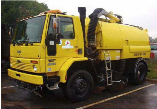
Figure 3.3-4: Bridge sweeping equipment: Allianz Johnston VT650 sweeper.
