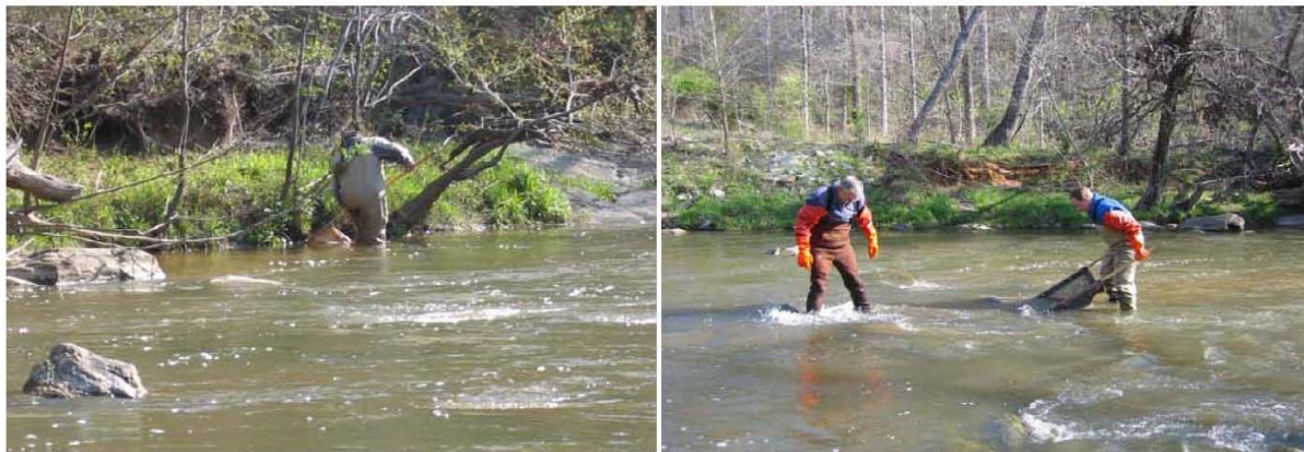
Figure 3.4-5: Benthic sampling techniques: sweep net (left) and kick net (right).
