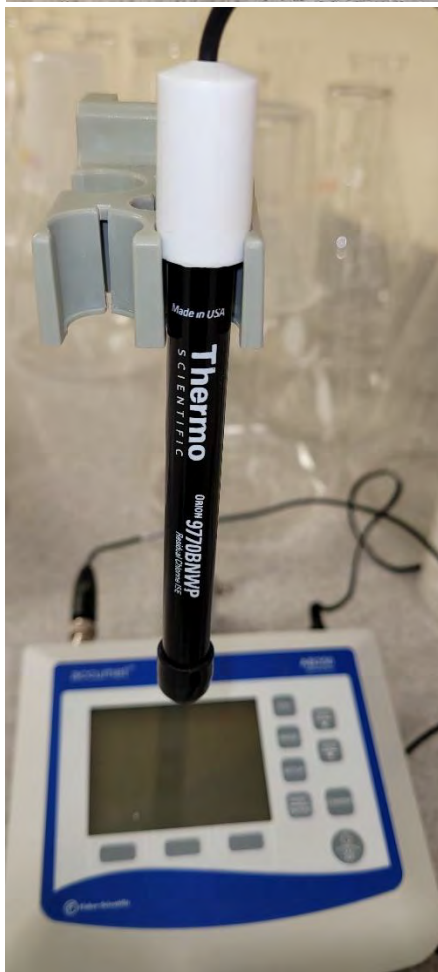
SOP-C8: Total residual chlorine meter/probe and reagents/standards
