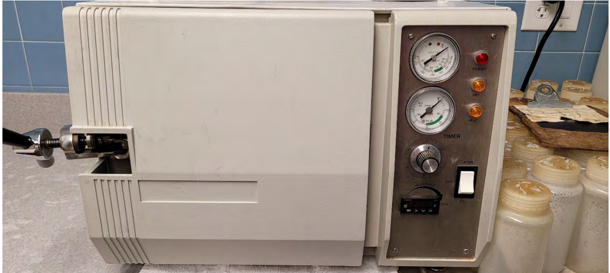
SOP-B1: Autoclave (used for algae media sterilization)
