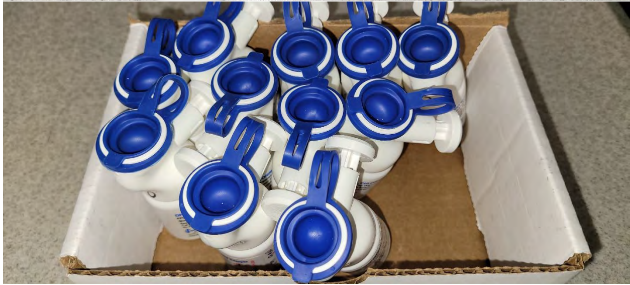
SOP-C8: Total residual chlorine DPD used for screening
